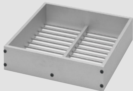
Grid sieve made in accordance with DIN EN 933-3
